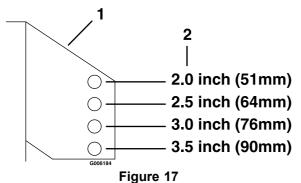
For cutting heights above 3.5 inches (90 mm) use the bottom hole. The rollers will still be effective against scalping.
